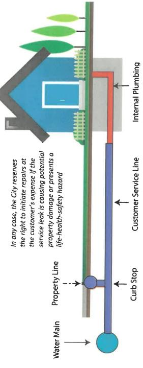
If a service leak can be stopped by closing the curb stop, the customer has the choice of having the City repair the service up to a reasonable distance outside the foundation wall of the structure or they may perform the repair on their own. Water may be turned off until repairs to the service line are certified by the City.
