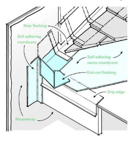
Because sidewall flashing must handle a large volume of water, one of the most critical flashing details occurs where the roof-wall junction terminates. To deflect water from the siding, install a kick-out in the corner.
