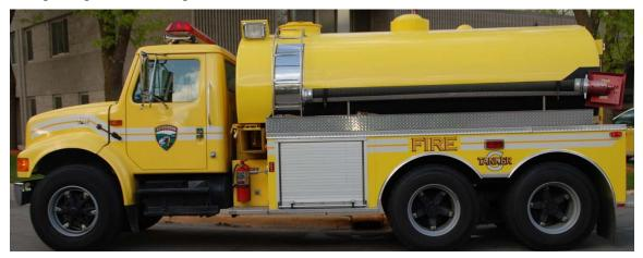
**Engine 7** was delivered on February 14, 2008. It is a 2007 General Fire Safety Apparatus built in Wyoming, MN. It features a 1250 gallon per minute pump, carries 1000 gallons of water, and 30 gallons of Class A firefighting foam. It features LED emergency and compartment lighting and a FoamPro Class A firefighting foam system and it carries a second Jaws of Life for extrications. Engine 7 has ability to transport up to six firefighters. Engine 7 is the first out engine.
