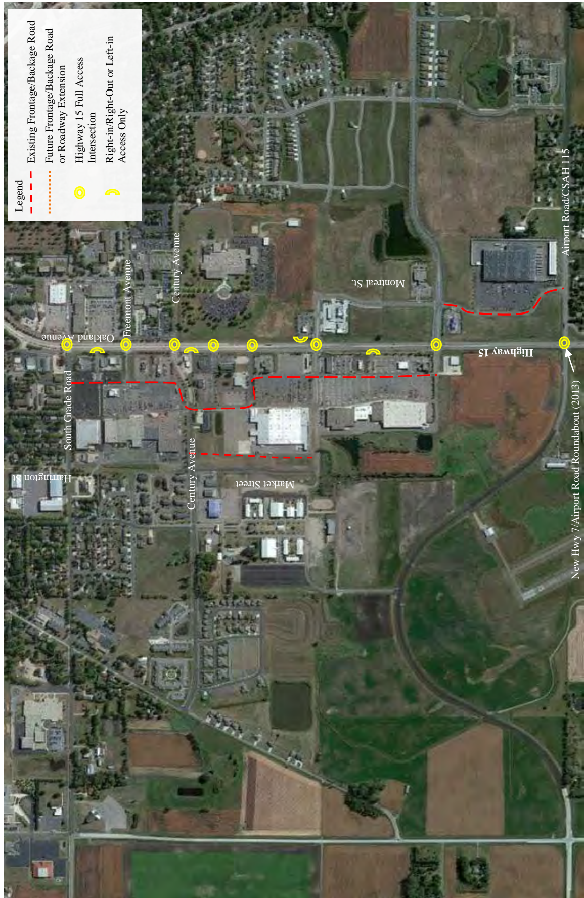
Figure 14 – Highway 15 South – Frontage/Backage Road System
